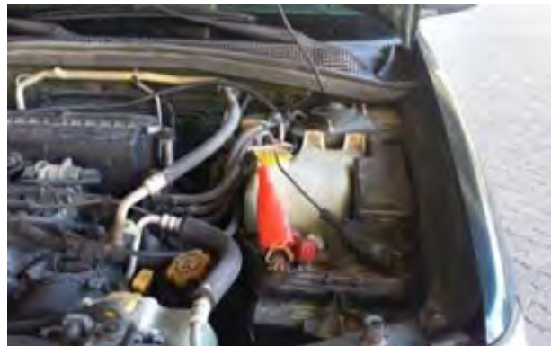
Figure 12. Power Cable Connection in PEMS Installation.
