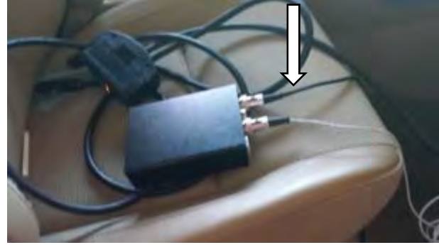
Figure 14. Connection of RPM Cable with Sensor Connector Box (Black Wire)
