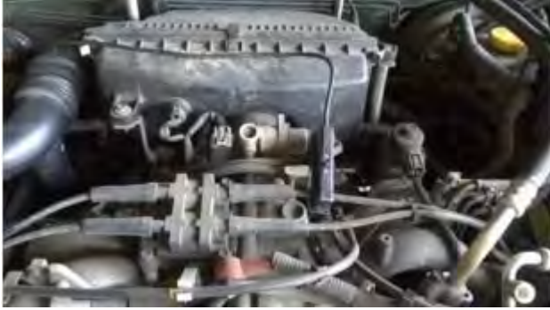
Figure 13. RPM Connection with the Black Wire of Test Vehicles Engine
