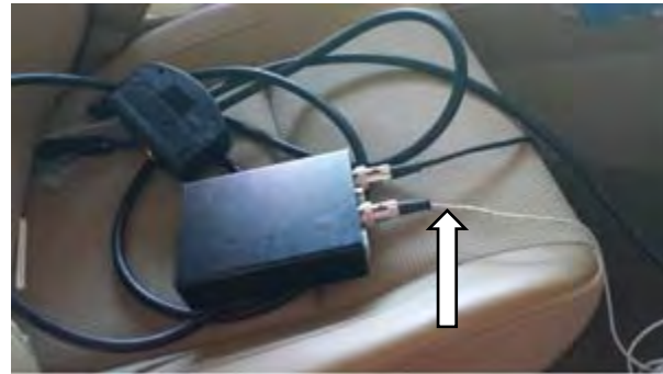
Figure 16. Connection of Temperature Sensor Cable with Sensor Connector Box (White Wire)
