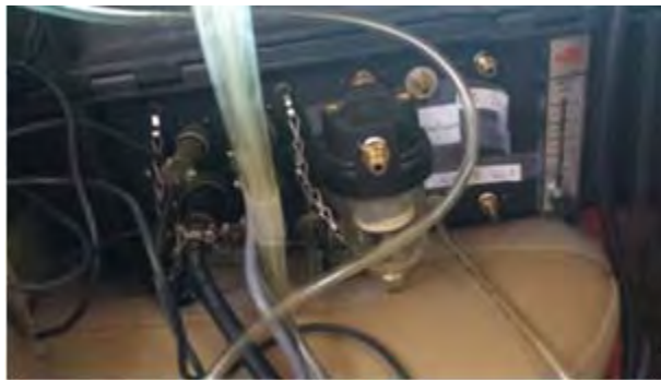
Figure 19. Connection of Pressure Cable with PEMS Computer.
