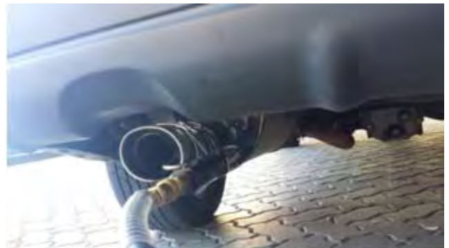
Figure 21. Installation with the Tailpipe of the Test Vehicle Other Connections.
