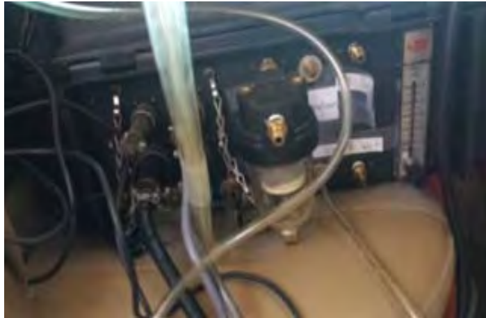
Figure 22. Other End of the Exhaust Cable is Connected to the H 2 O Condensation Bowl.
