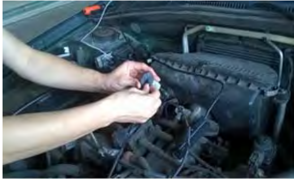
Figure 18. Installation of Two Heads of the Pressure Cable.
