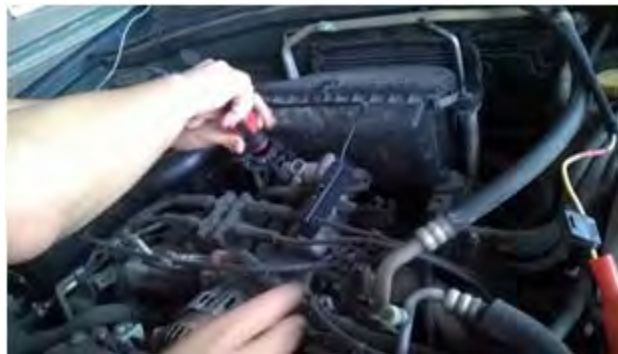
Figure 17. Unscrewing the Pressure Port of Test Vehicle Engine.
